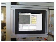
SensoWeb is called up by simply entering the IP address of the sensor to be monitored in the browser. The full-screen view of live pictures can be activated via the appropriate browser function or by entering a direct link. Web monitoring can also be deactivated if it is not used.
